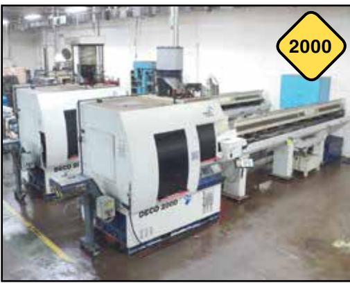
(2) Tornos Bechler Mdl. DECO 20/25.4 CNC Swiss Type Automatic Screw Machines, 10-Axis, 25.4mm
