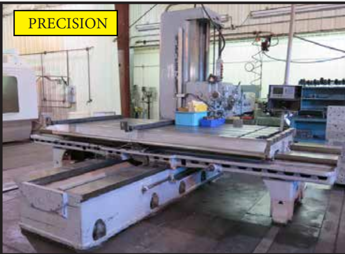
Giddings & Lewis mdl. 340-T Horizontal Boring Mill s/n 150-253-57 w/ 110" x 48" x 60" Travels, 26" Quill Travel, Acu-Rite DRO, 10-1300 RPM, 4" Spindle, Power Feeds, 48" x 122" Table
