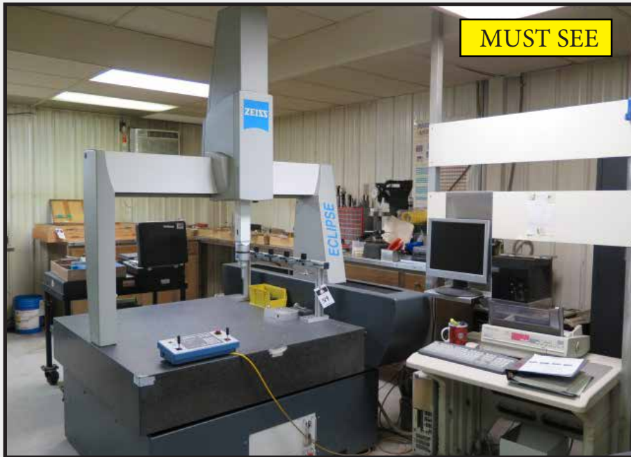
1997 Zeiss ECLIPSE 4040 CMM Machine s/n CMM970203058 w/ Zeiss ST Dynamic Probe, 5-Station Automatic Probe Changer, 28" x 40" x 20" Work Envelope, 36" x 52" Granite Table, Zeiss Joystick Controller, 0.00008" Repeatability, 0.00002" Resolution, U-Soft Software
