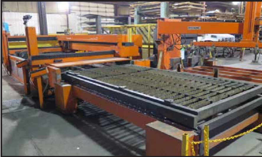
1995 Bystronic BYSTAR 3015 2-Pallet CNC Laser Contour Cutting Machine s/n 341 w/ Bystronic Controls, 5' x 10' Cap, Bystronic Automatic Vacuum Sheet Loading System, Rotary Tube Option with 12" 4-Jaw Chuck and 5 3/4" Thru Bore, Bystronic Laser BTL2800 Turbo 2800 Watt Laser Source, Koolant Koolers Cooling System, Lazervac 2442 Dust Collection System
