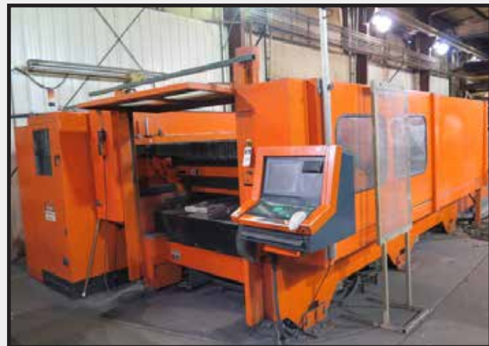
1998 Bystronic "By Sprint 2512.2" 2-Pallet CNC Laser Contour Cutting Machine s/n 60 w/ Bystronic Controls, 6-Pallet Shuttle System, 50" x 122" Pallets, Bystronic Automatic Vacuum Sheet Loading System, Bystronic Laser BTL1800 1800 Watt Laser Source, Koolant Koolers Cooling Unit, laser was just recently fully refurbished and cleaned.
