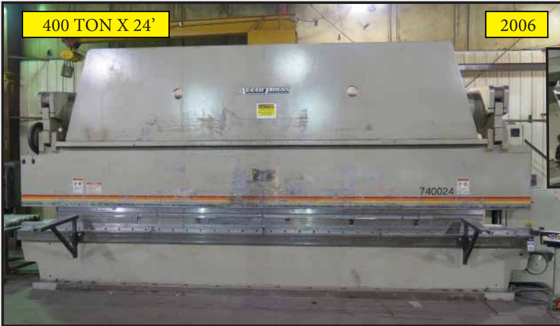
2006 Accurpress mdl. 740024 400 Ton x 24' CNC Hydraulic Press Brake s/n 8724 w/ Accurpress ETS Pedestal Controls, 24' Bed Length, 20' Between Uprights, 10 1/4" Throat
