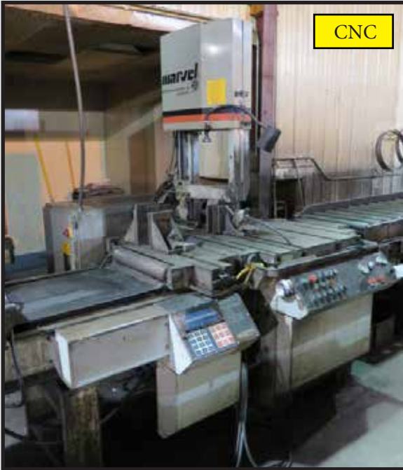
Armstrong - Blum / Marvel Series 87A11PC CNC 18" Vertical Miter Band Saw s/n E-469111PC w/ Marvel Controls, Hydraulic Clamping and Feeds, Coolant, Conveyors
