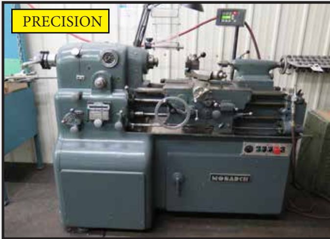
Monarch mdl. EE Tool Makers Lathe s/n EE-45265 w/ 0-4000 Digitally Controlled RPM, Taper Attachment, Inch Threading, Tailstock, 5C Collet Closer, 6" 3-Jaw Chuck
