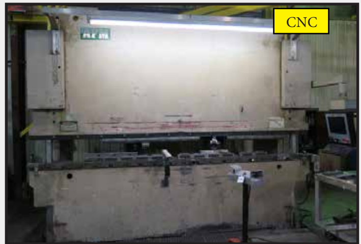
AFM mdl. EP13-220 220 Ton x 13' CNC Hydraulic Press Brake s/n CHPB/9-71439 w/ PC800 controlled Back Gaging, 13'4" Bed Length, 135 1/2" Between Uprights, 16" Throat
